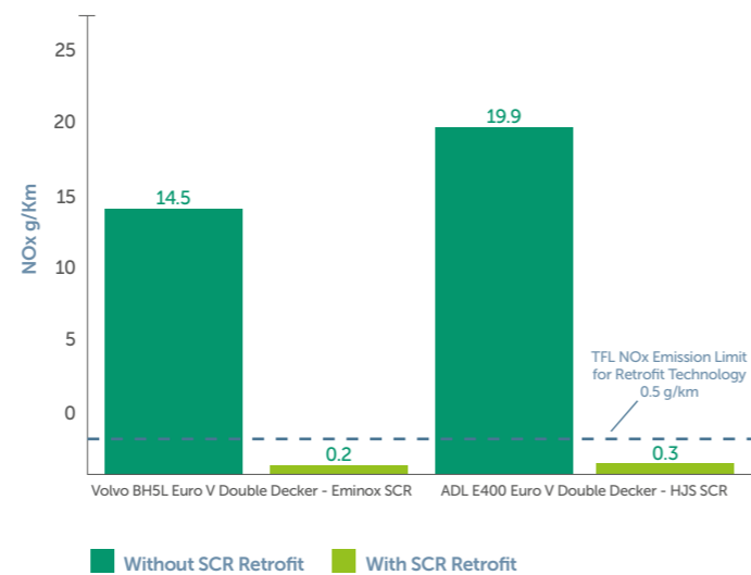
Diagram 3: Vehicle Emissions Testing Results - NO x Emissions for TfL Euro V Buses Before and After SCR Retrofit
